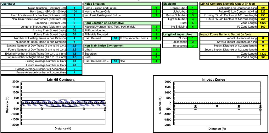
Instruction sheet for using the FRA horn noise model.
