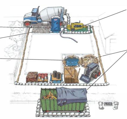
Prevent equipment fluid leaks onto ground by placing drip pans or plastic tarps under equipment. Repair equipment as necessary.
