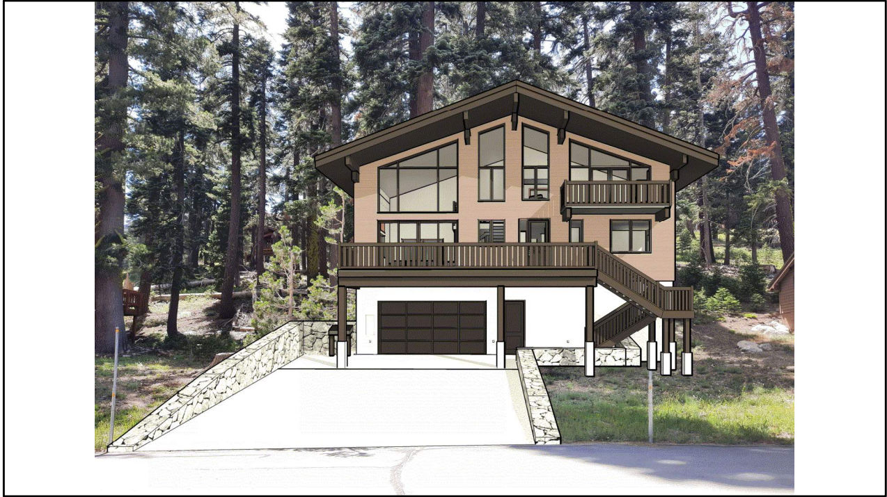
Side walls on the driveway are low as possible, scaled humanely using dry stacked stone
