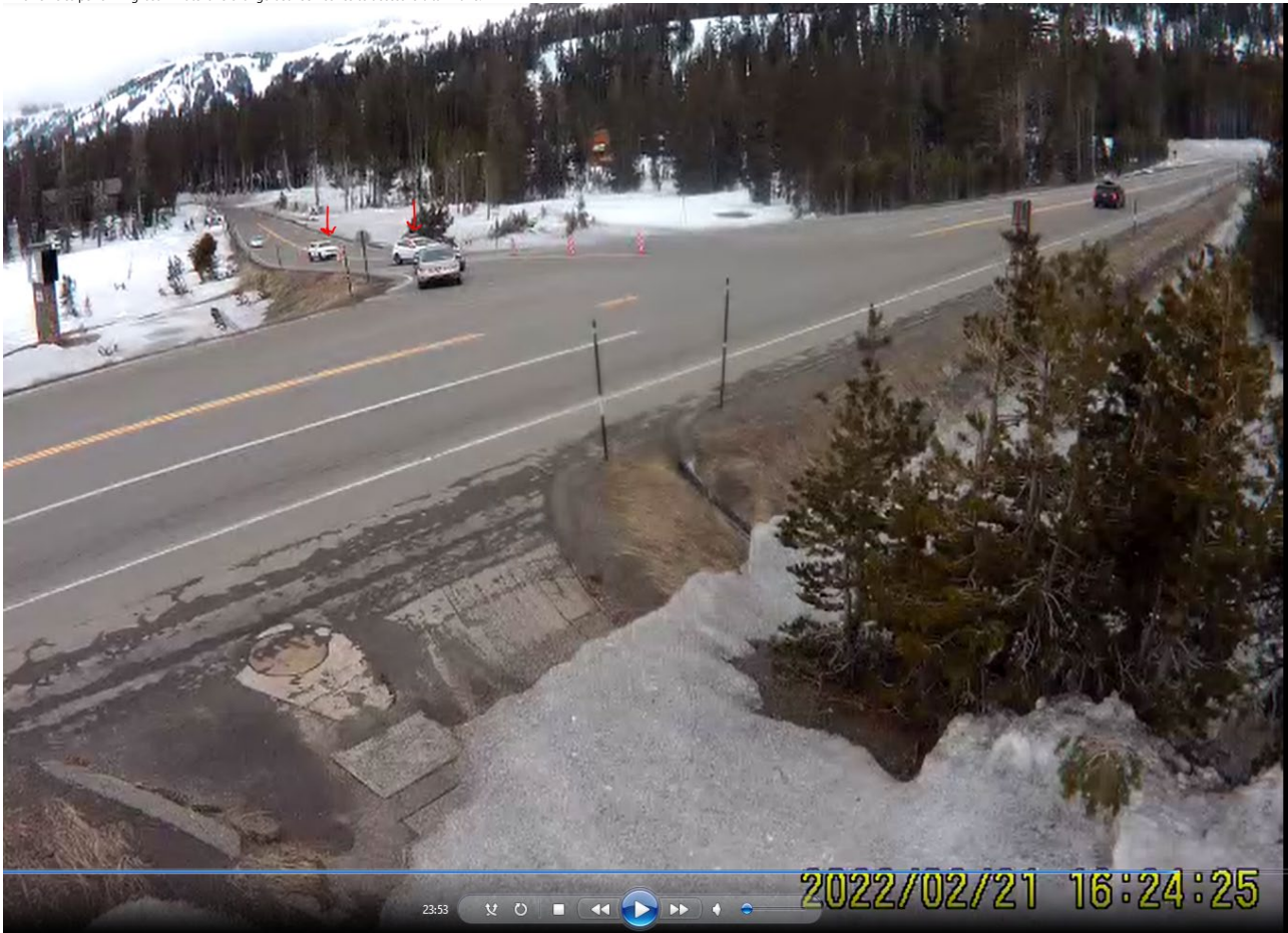
Two vehicles performing last minute lane change between cones to access left-turn lane.
