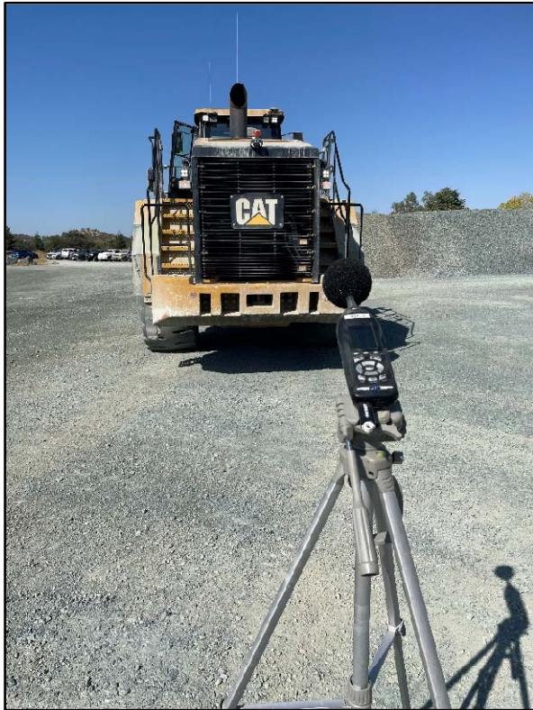
Figure 12 – Backup “beeper” warning device test
