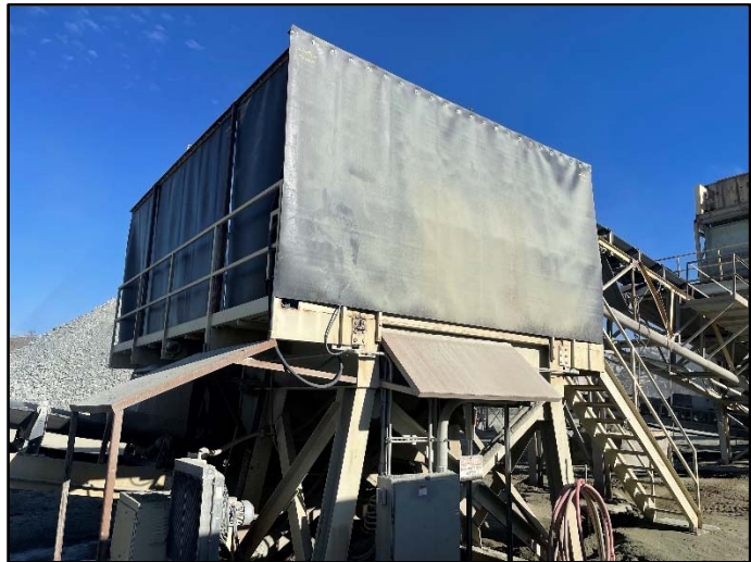
Figure 10 – Crusher GP500 after acoustic curtain installation
