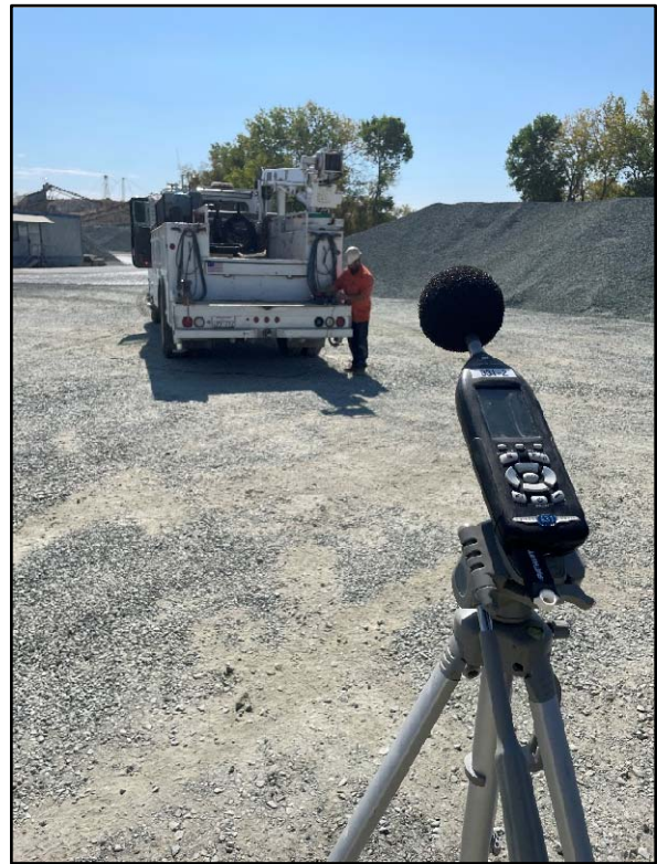
Figure 13 – Broadband backup warning device test
