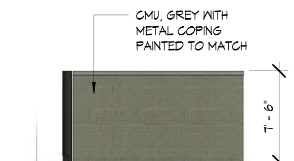
11 TRASH ENCLOSURE SIDE ELEVATION 1/8" = 1'-0"
