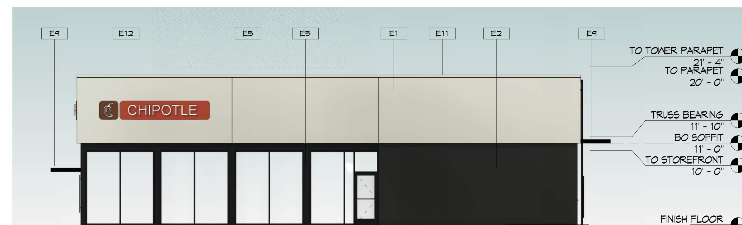
2 EAST EXTERIOR ELEVATION 1/8" = 1'-0"
