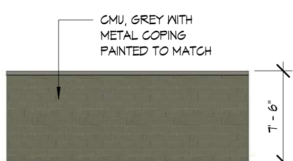
12 TRASH ENCLOSURE REAR ELEVATION 1/8" = 1'-0"
