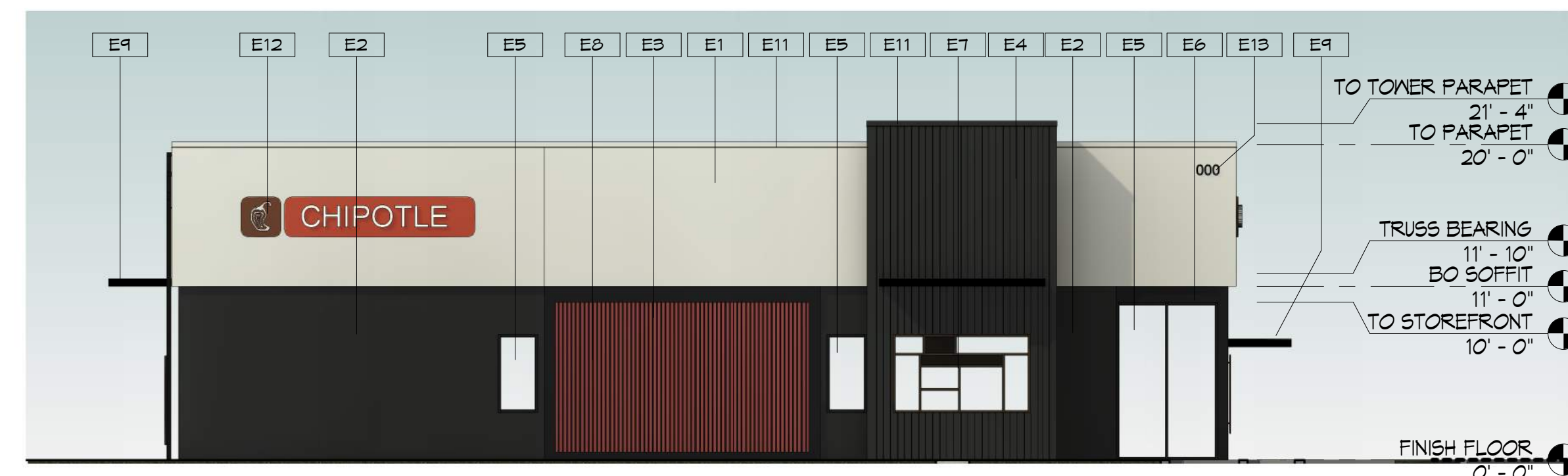
4 WEST EXTERIOR ELEVATION 1/8" = 1'-0"
