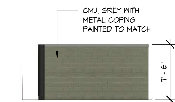
11 TRASH ENCLOSURE SIDE ELEVATION 1/8" = 1'-0"
