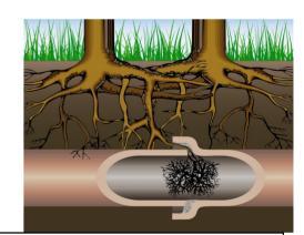
8. Plant only grass over and near your septic system. Roots from nearby trees and shrubs might clog and damage the system. Also, do not apply manure or fertilizers over the drainfield.
